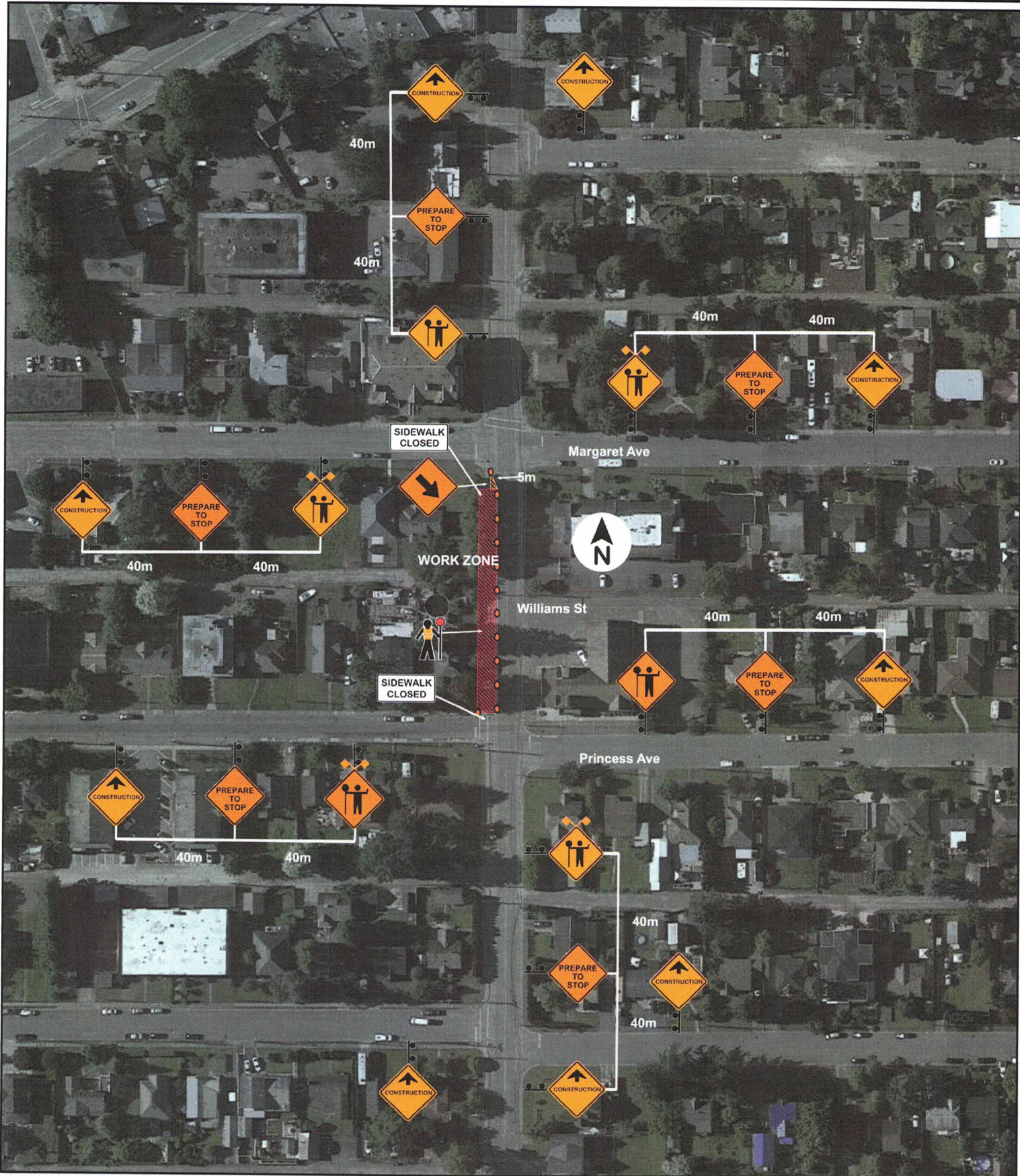
Figure 7.5: Work on Shoulder - Short and Long Duration TCP on site to assist with vehicles, pedestrians, bicyclists and all others
